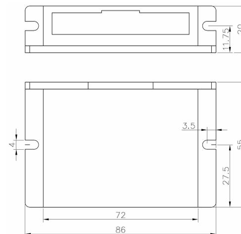
Figure 1: Mechanical dimensions
