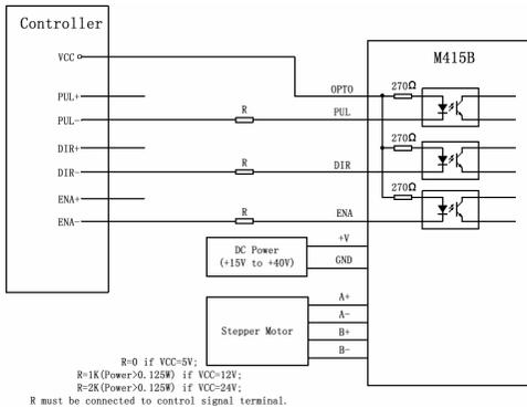
Figure 10: Typical connection with difference controller
