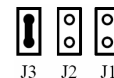
(c) J1, J2 open circuit, J3 short circuit CW/CCW mode and active at low level (The fixed level)
