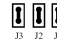
(d) J1, J2, J3 short circuit CW/CCW mode and active at high level (The fixed level)
