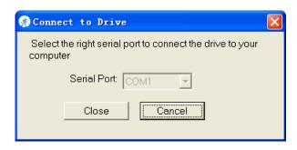
**Connect to Drive** window appears every time you open ProTuner. You can also open it by clicking **Drive->Connect** any time. Select the serial port and click on the **Connect** button. The software will try to connect to the drive and read the settings. It may take several minutes. Please wait.
