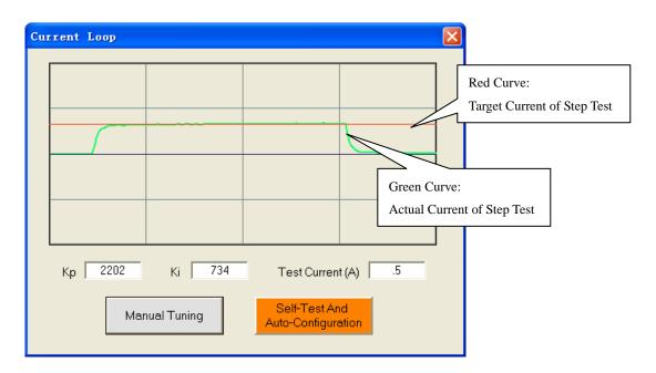
Click **Drive->Current Loop** to open the current loop tuning window. You can adjust the Kp (proportional gain) and Ki (integral gain) in this window. These parameters should be tuned before normal operation.
