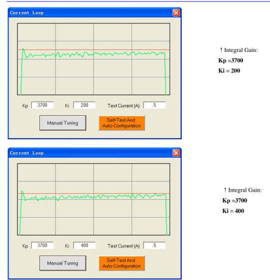
**Step 5:** The current loop tuning is basically finished. You can continue to adjust Kp and Ki for better performance. Now the updated Kp and Ki is just stored in the driver's RAM. They will be lost when we power off the driver. **Don't forget to click Drive->Download To Drive to store the changed value to the drive's EEPROM.**
